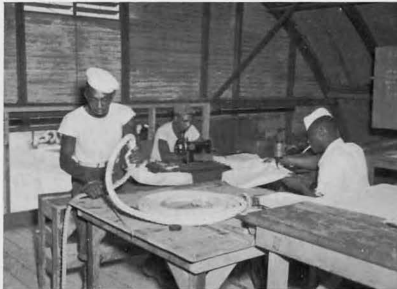
One of the most useful shops in a Construction Battalion is the Sail Loft. All canvas work, such as tent repair, tarpaulins, truck and jeep tops, rope work etc., saves a lot of equipment and material. Large sewing machine is a salvaged Jap machine.
